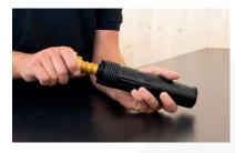
Tighten the chamber element manually using the multi-tool. The fire tube and the end surface of the inner core must flush
