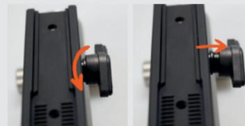
1. Activate the locking levers by turning them 10° clockwise or counter clockwise and pull away from the mount body. Loosen the clamp units by turning the locking levers counter clockwise until the mount can be placed on the prism.
